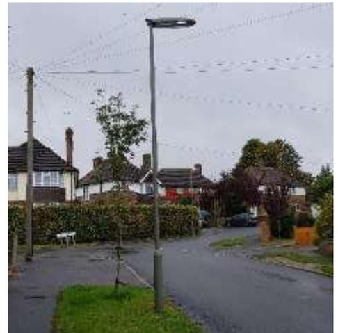
*Picture 3 - Rowan tree planted under telephone cables and too close to a street lighting column – this will cause issues in the near future.*
